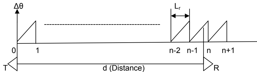
Fig. 3. Relation between d = c \cdot \Delta t and d = (n-1) \cdot L_r + (\Delta\theta/2\pi) \cdot L_r .
